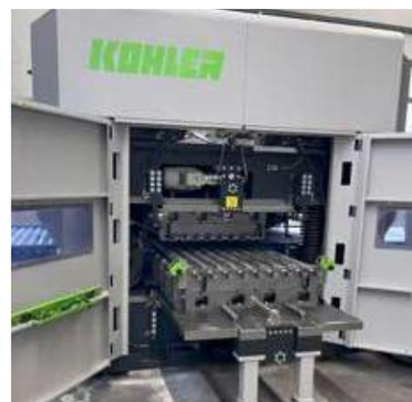
The Peak Performer ensures level and low-tension metal sheets.
